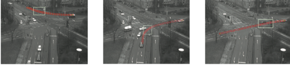
Figure 6: An example vehicle trajectories : right turn (left panel), left turn (middle panel) and straight line (right panel).
